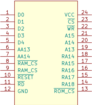
Figure D.13: MBC1 (Sharp SOP24-P-450) [6]
